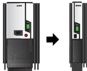
\* When only 1 car is connected, charger provides the maximum required power, when 2 cars are connected (one in AC and another in DC) the charger splits the maximum output power between 2 cars. \*\* Only 1 DC car can be charged at one time, even though there is more than one DC connector. Queuing is available in AC and CHAdeMO. Maximum 2 User Unit can be used per QuickCharger.
