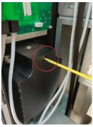
• Loosen or tighten the set screw on top to determine the tightness of the CCS2 socket.
