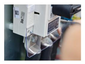
Connect the ground (PE) to the distribution block on the right of the EV Ultra, using an 8 mm hex wrench. Tighten it to **25 Nm**.
