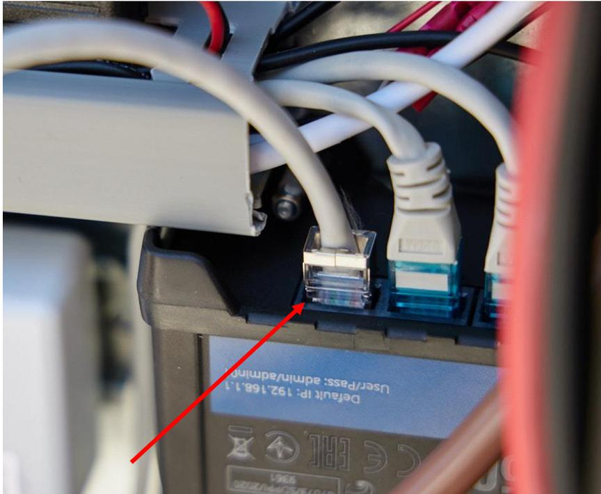
The Teltonika router creates a small, private network within the EV Ultra to provide network connectivity for all components. This private network is created within the subnet 192.168.37.0.
