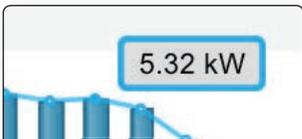
Tool tip display when the cursor is over the graph. Displays the total of the individual values of the power inverters.
